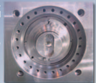
Prototype AB3 TM Valve with end caps removed
