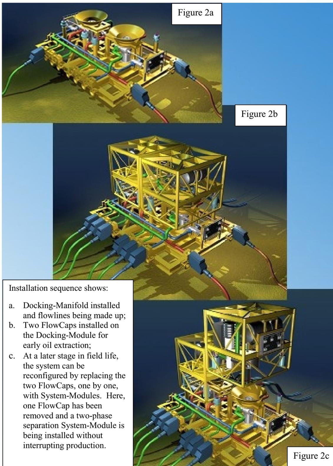
**Figure 2 – AlphaPRIME™ CPU: Installation Sequence**
