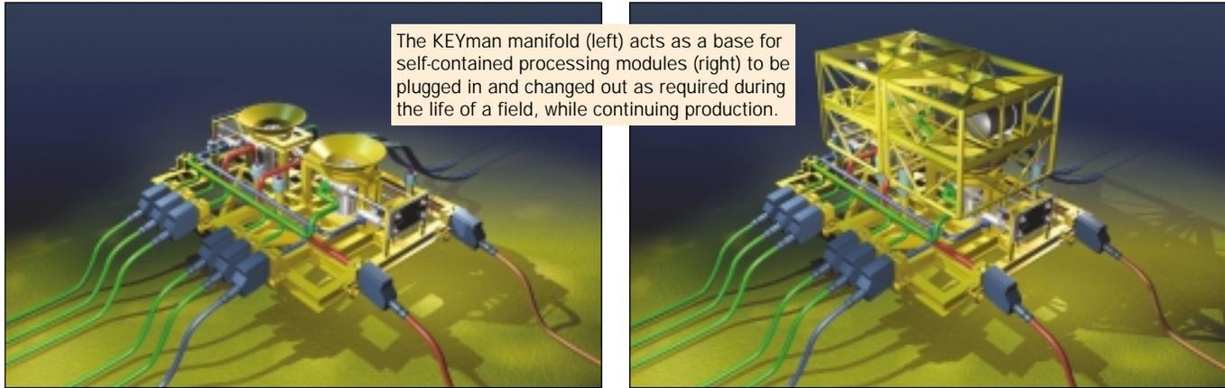
The KEYman manifold (left) acts as a base for self-contained processing modules (right) to be plugged in and changed out as required during the life of a field, while continuing production.
